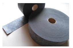
Material description:Sealing material based on ethylene propylene diene monomer<br/>rubber, with excellent resistance against heat, ozone, oxygen and<br/>other atmospheric influences. EPDM possesses outstanding<br/>ageing resistance, good resistance against acids and caustic or<br/>base solutions, is alcohol resistant, and remains elastic and<br/>flexible throughout the temperature spectrum.Typical applications:The ERDM scaling strip is used mainly for airtight, waterproof and
